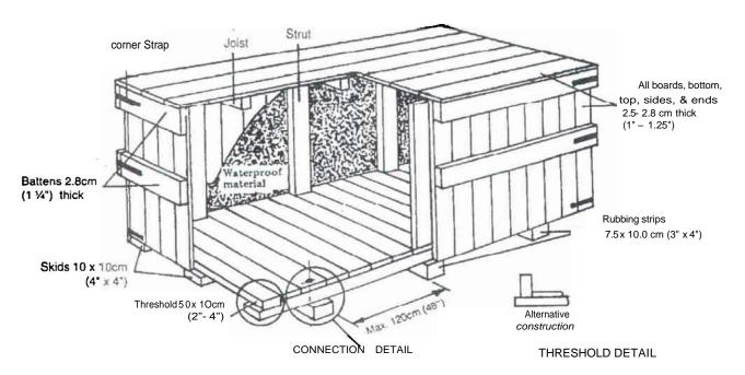
Notes: 1. Bolt connections are required when point loads will result in distortion of the base during lifting by sling if required, adopt SOLT CONNECTION DETAIL shown in BOX TYPE 3.
