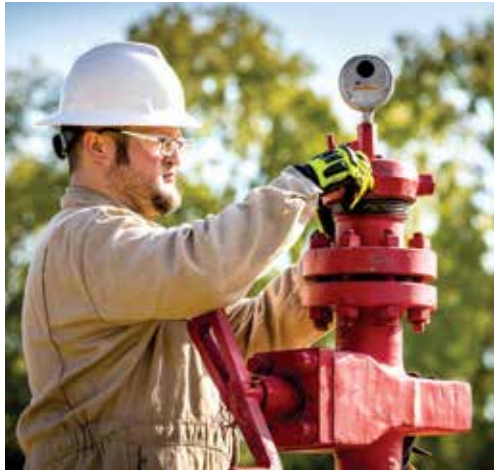
Engineer Robert Adams prepares to test new instrumentation in the test well. The well, on-site at the Aramco Research Center-Houston, is outfitted with 32 strands of fiber optic cable and arrays of geophones and hydrophones to evaluate new fiber optic sensing methods.
