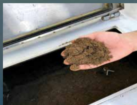
Food and garden waste at Berri Gas Plant is tossed into a steel-encased compost machine, where it is converted into high-quality organic fertilizer in approximately 24 hours.
