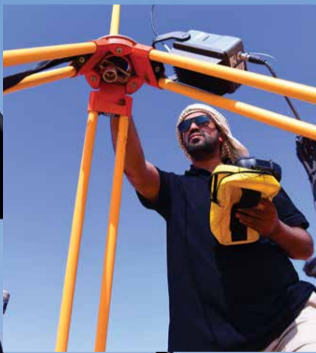
Sultan A. Marri calibrates the GPS coordinate data receiver at a reference scan point. The reference survey points associated with the global coordinate system are a main pillar in obtaining highly accurate local data, and these points scattered in many regions, are built and measured across several private and governmental bodies to serve the purposes of the high precision survey. Marri holds a bachelor's degree in Surveying and Cartography from the University of Newcastle, U.K.
