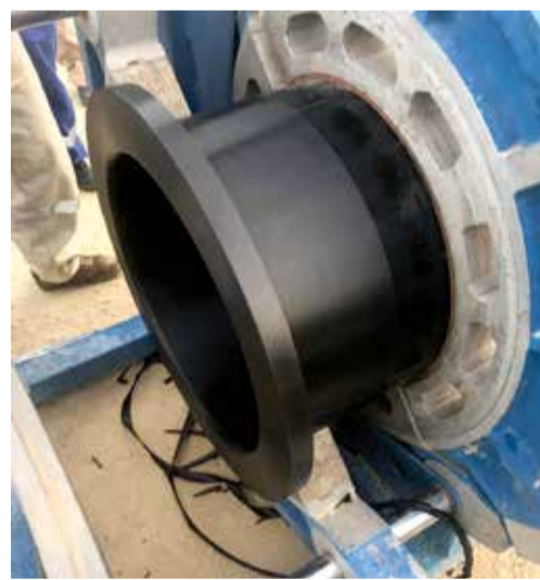
The Manifa Producing Department has teamed up with the Consulting Services Department to deploy critical nonmetallic technologies in its pipeline network such as raised temperature, high-density polyethylene lining.
