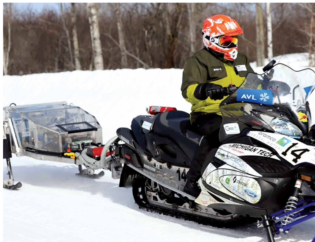
A member of the MTU team chews up a little snow along one of the Michigan trails, demonstrating the team's success in developing a clean snowmobile engine. The attached trailer houses an in-use customized analyzer to measure emissions. Aramco served as a partnering sponsor of the MTU team.
