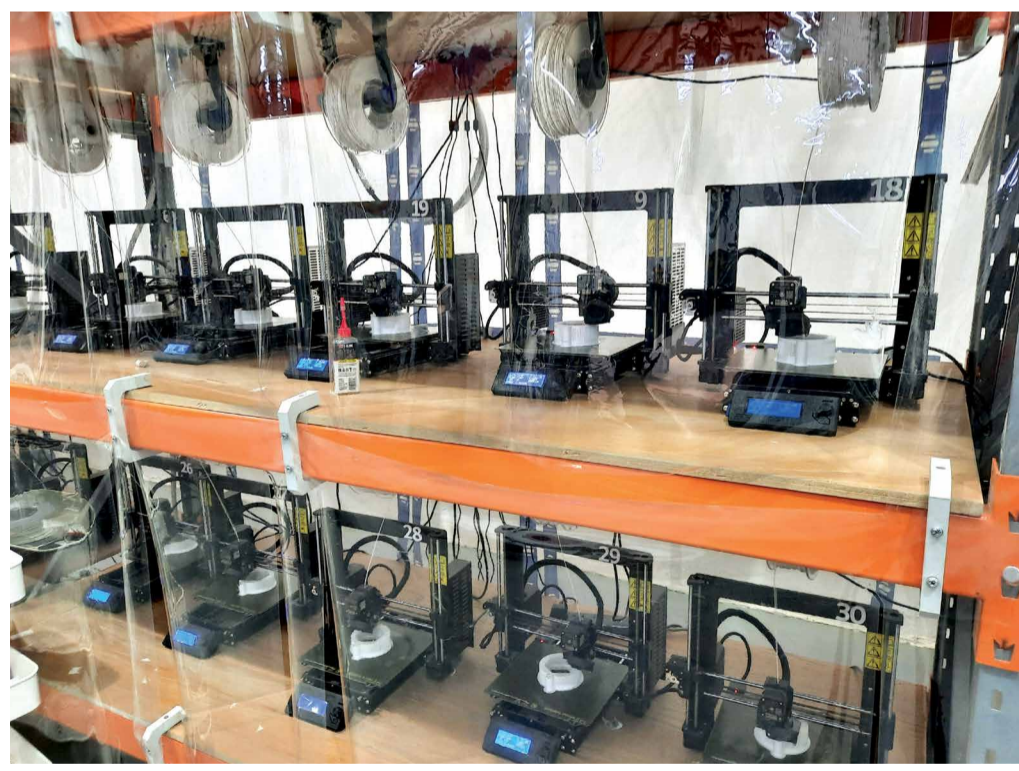
3-D printing the nonmetallic laterals using multiple printers.
