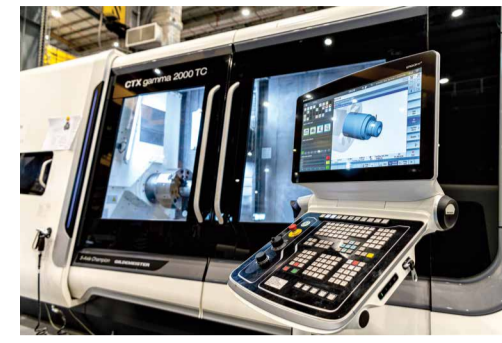
Top: The new MSSD shop in Ju'aymah includes advanced tools, such as this five-axis milling machine, which makes use of computer numerical control technologies to manufacture replacement parts in only hours. Left: Technicians Chris D. Nablo (left) and Sajjad A. Alzayer from the Mechanical Services Shops Department in Ju'aymah are machining the bearing seal in preparation for alignment and repair of a load gear box, using a new Computer Numerical Control Horizontal Boring machine.
