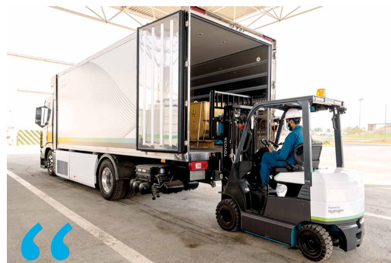
For the first time in KSA, a shipment is loaded onto a hydrogen truck with a hydrogen-powered forklift. (Photo: Ahmad El Itani/MPD)
