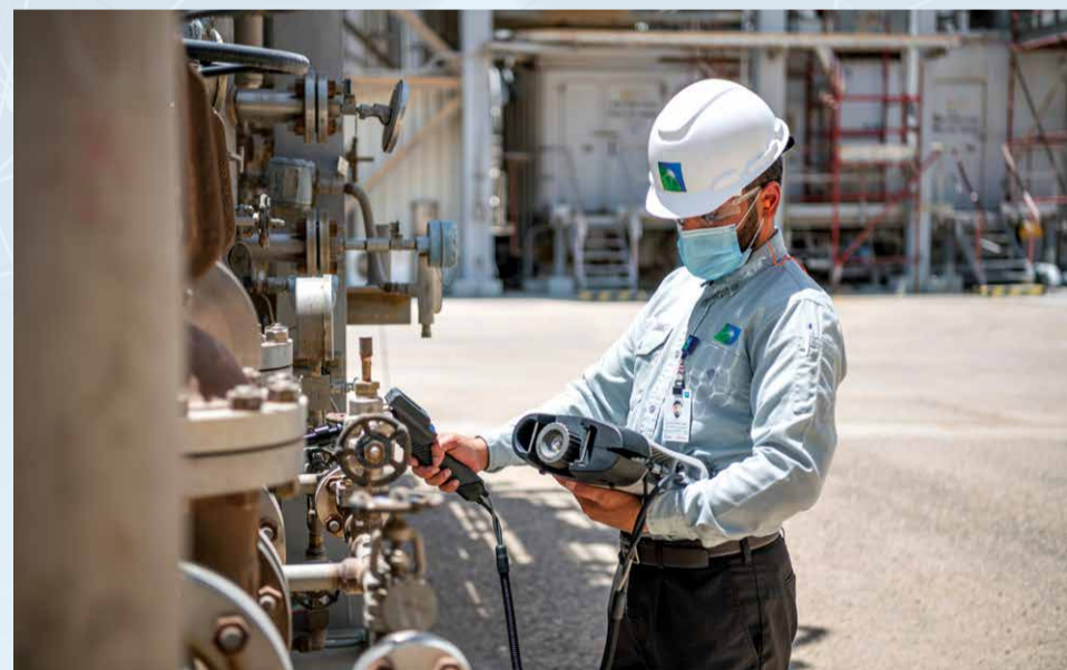
Operators provide a front-line check on fugitive leaks, and supervising operator Mohammad A. Zahrani checks valves at Abqaiq Plants cogeneration system.
