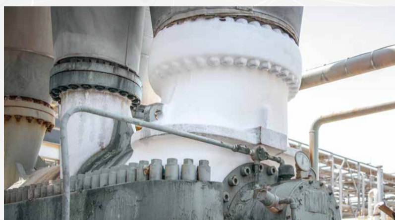
Working with technology makes for a lower carbon, more efficient, and safer operation, and in real-time, process engineer Turkey S. Alshuhail and operations shift superintendent Bdah F. Hajri examine thermal images monitoring the 1,200 degree Celsius metal skin temperature of Shedgum's sulfur recovery plant's refractory-lined reaction furnace to proactively identify any defects or hot spots requiring immediate isolation and repair.
