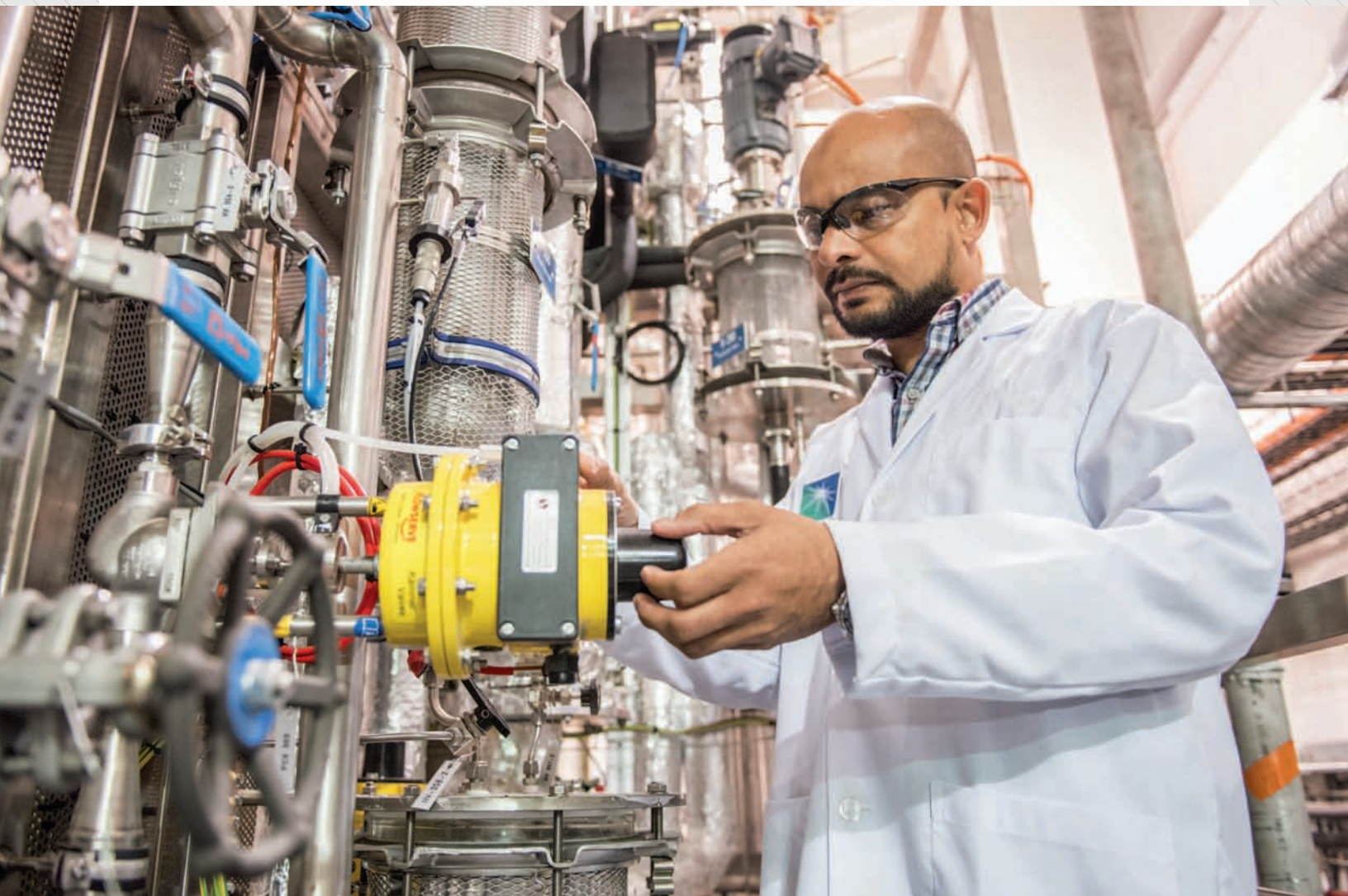
Scientist Kareemuddin M. Shaikh checks the pressure control valve for the pilot plant used for one of the crude to chemicals technologies.
