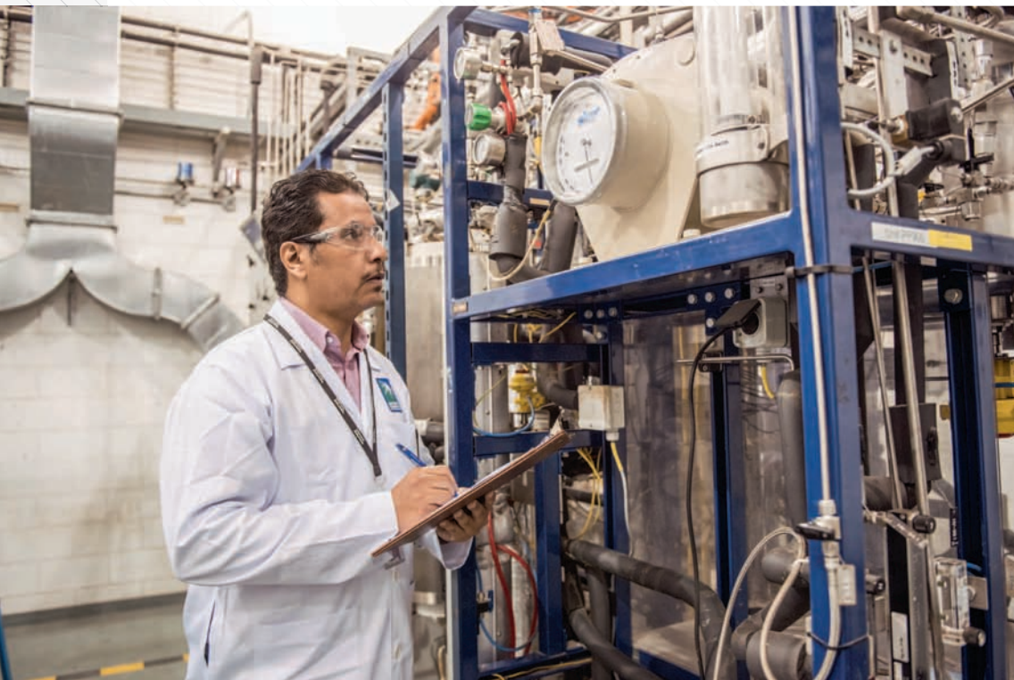
At one of the C2C laboratories, lab technician Duhaiman U. Yami monitors the wet test gas meter on a pilot plant for the crude conditioning step of the Thermal Crude to Chemicals research stream.
