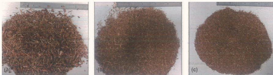
Fig. 3 ARC Eco-fibers prepared using deceased date trees available as date palm industry waste: (a) ARC Eco-fiber C, (b) ARC Eco-fiber M, and (c) ARC Eco-fiber F.
