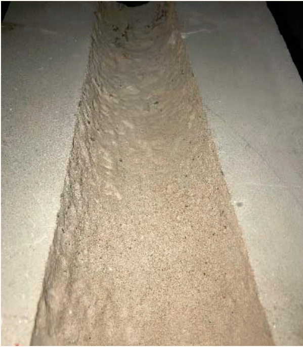
Fig. 17 Laser perforation of a large sample, 4" in diameter and 24" deep.
