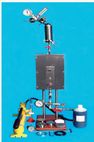
Fig. 6 PPT apparatus and the 2-mm slotted disc used for testing the ARC plug.
