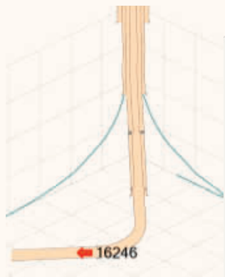
Fig. 11 Well-9 simulation result lockup depth without FAPT.
