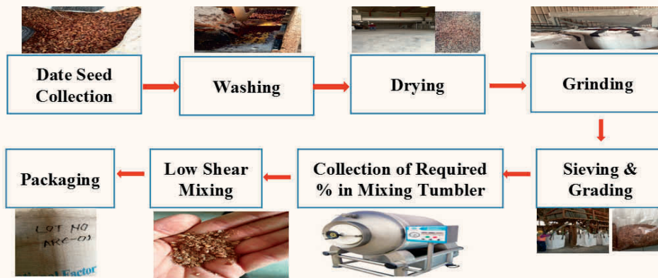
Fig. 4 Block diagram showing the ARC plug manufacturing process, a sized particulate LCM.
