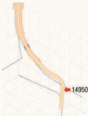
Fig. 12 Well-10 simulation result lockup depth without FAPT.
