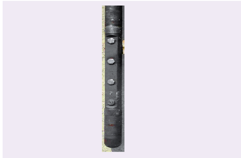
Fig. 5 The HPJN with orifices on the same plane.
