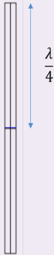
Fig. 2 Schematic of the Tx and Rx. Each arm has the length of one-quarter of a wavelength. The highlighted section represents the gap between the arms.
