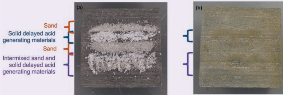
Fig. 11 Photos of the Eagle Ford outcrop Sample III for Experiment #3: (a) surface of the half core packed with solid delayed acid generating materials and 100 mesh sand in four patterns before being put into the coreflood setup; and (b) surface of the core plug after being retrieved from the coreflood experiment.
