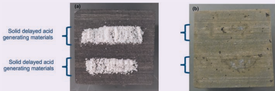
Fig. 8 Photos of the Eagle Ford outcrop Sample II for Experiment #2: (a) Surface of the half core packed with solid delayed acid generating materials alone before putting into the coreflood setup; and (b) surface of the core plug after being retrieved from the coreflood experiment.
