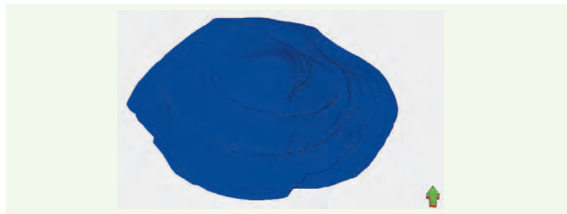
Fig. 6 A 3D illustration of the isosurface enclosing the region of influence for s = +2 after 31 hours around Well-C.
