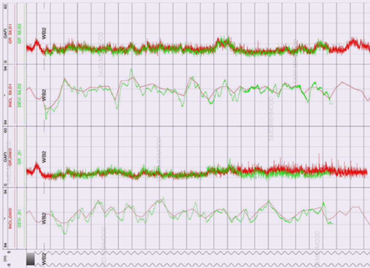
Fig. 10 The gamma ray and deviation surveys for the MLT access confirmation.
