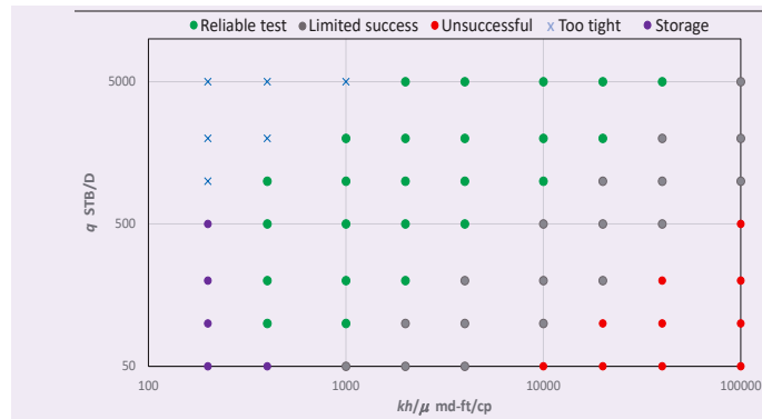
Fig. 13 A summary of probable valid tests under tidal effects with test durations of one hour to four hours.
