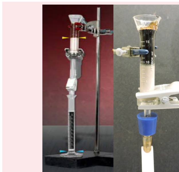
Fig. 1 The gravity drainage fluid recovery column apparatus used.
