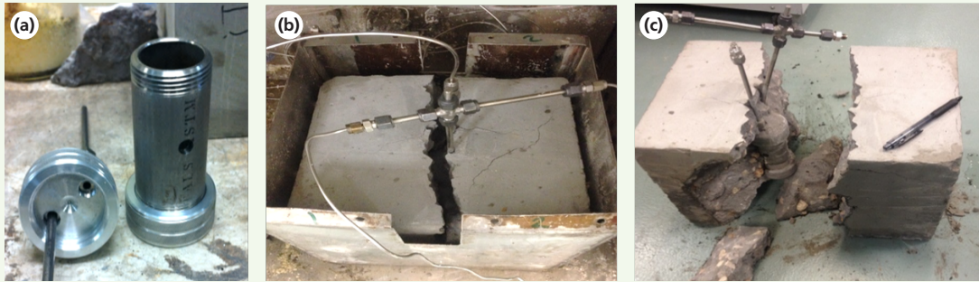
Fig. 7 (a) The pre-perforated casing, (b) and (c) post-reaction pulse of the portrait cement block sample.
