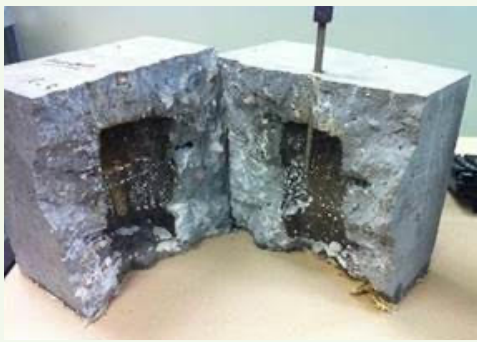
Fig. 8 Chemically pulsed fracturing in a cement block with four notches, simulating an open hole wellbore.
