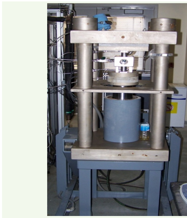
Fig. 3 The HPHT autoclave system, rated up to 20,000 psi and 500 °C.
