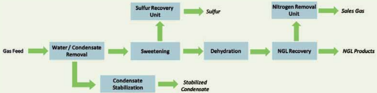
Fig. 1 A schematic of the different processes found in a typical gas plant.
