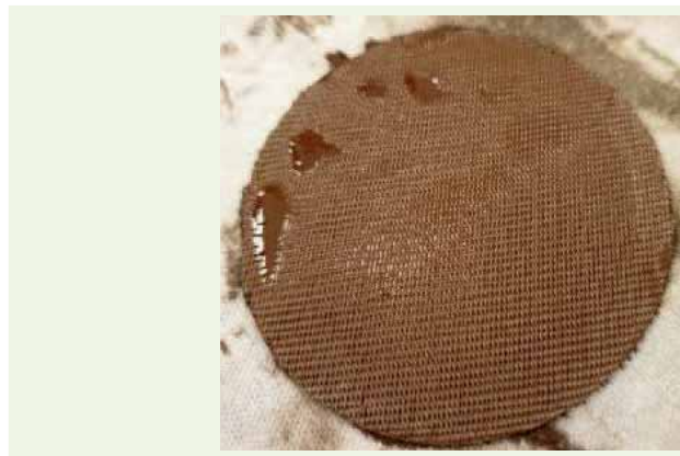
Fig. 8 The 250 \mu screen after PST, showing no residual buildup on the face of the coupon.
