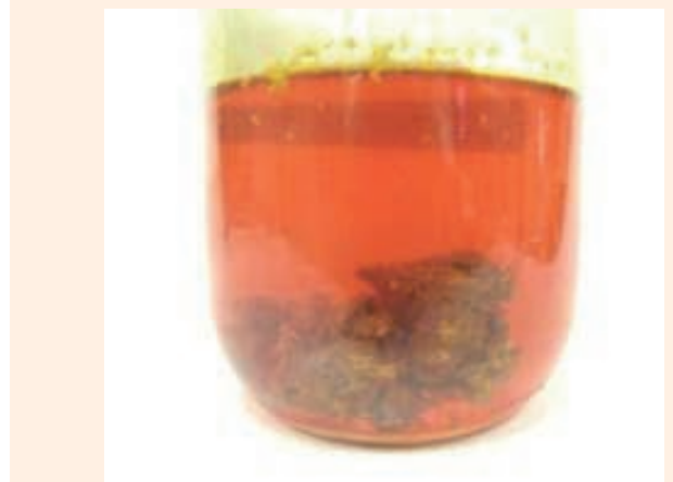
Fig. 3 The cross-linking of the amphoteric VES with corrosion products, Fe (III) forms sludge 10 .
