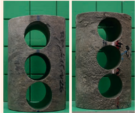
Fig. 1 Images of the reactive shale sections where the plugs were drilled horizontally to be used as samples.
