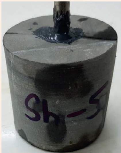
Fig. 4 A view of the prepared shale rock sample.
