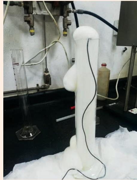
Fig. 5 Generation of the in situ foam by an activating reaction.
