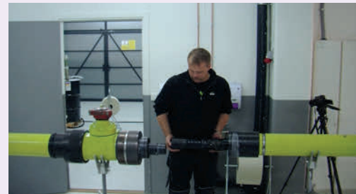
Fig. 1 An example of the full-scale e-DST qualification testing under simulated downhole conditions.
