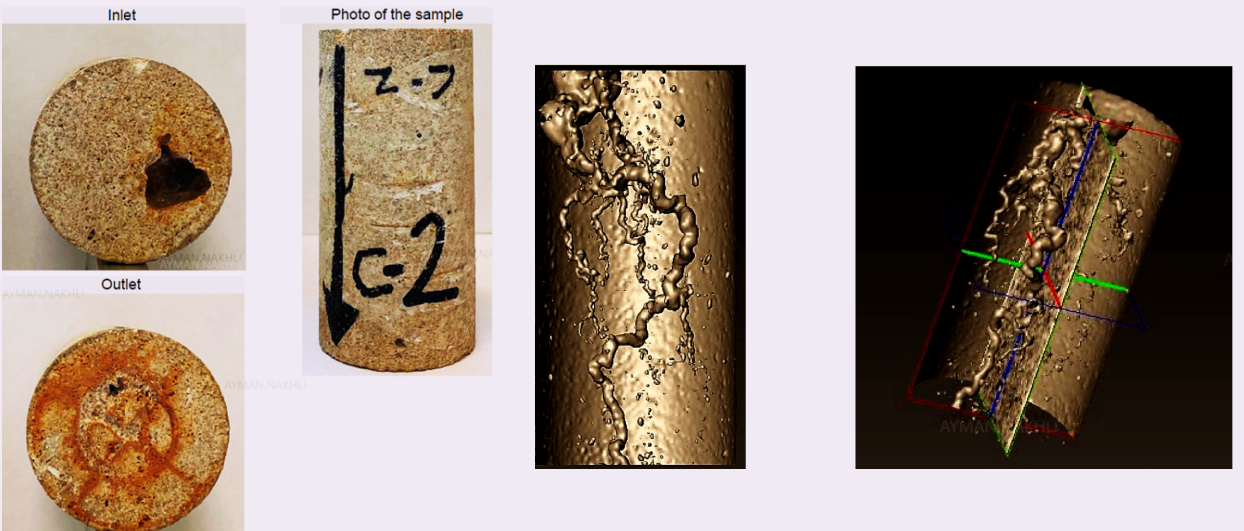
Fig. 11 The CT scan images of the carbonate core with in situ foam generating system post-treatment.
