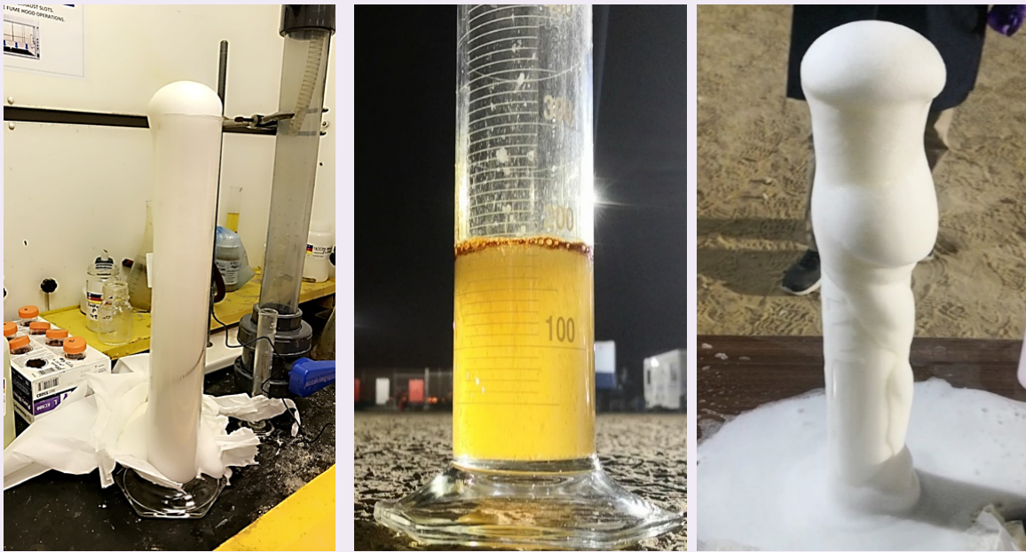
Fig. 12 The lab and field testing of an in situ foam generating system, expanding up to thirtyfold of the original fluid volume.
