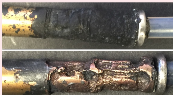
Fig. 7 The suspected heat effect (top) turned out to be H_2S corrosion (bottom).
