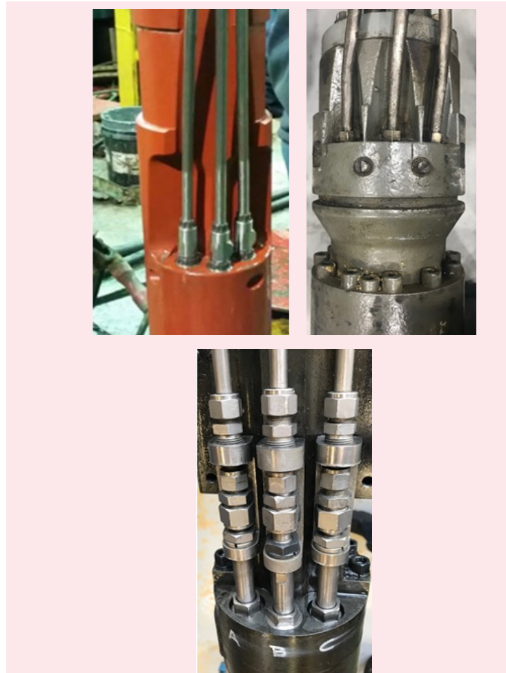
Fig. 16 Three different MLEs with metal-to-metal sealing technology.
