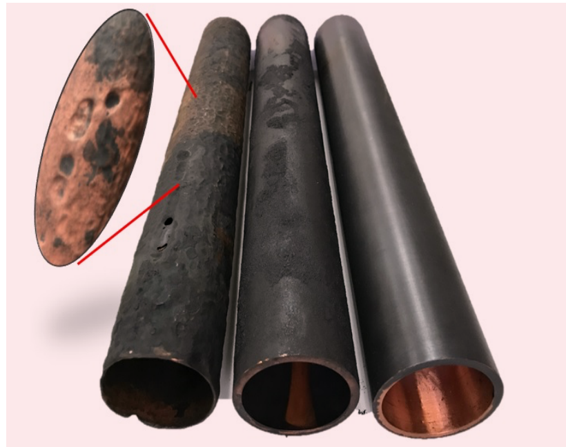
Fig. 18 A comparison of H_2S scavengers from a B/B/B seal showing H_2S corrosion progress from upper (left) to lower (right) bag chambers.
