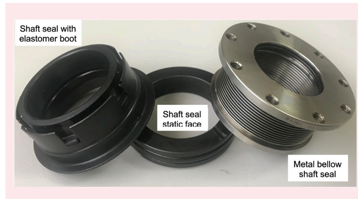
Fig. 19 A comparison of shaft face mechanical seals.
