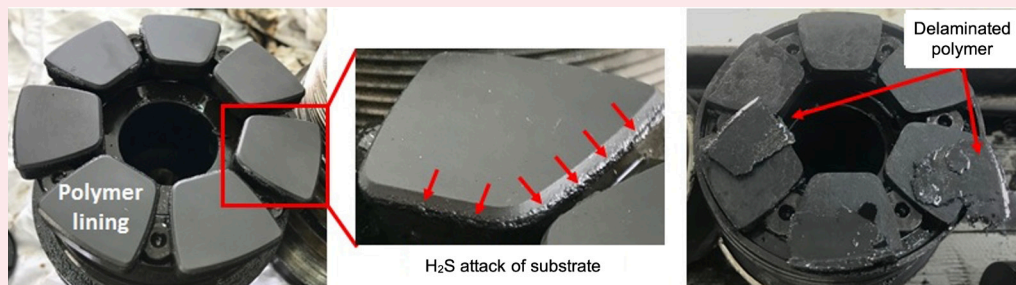
Fig. 13 The delamination of lining polymer in tilting pad thrust bearings initiated by H_2S corrosion of the bronze substrate.
