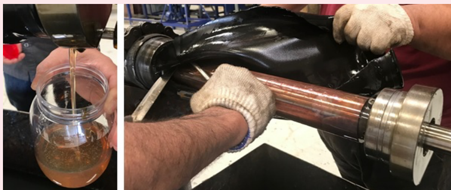
Fig. 17 Dielectric oil and H_2S scavenger from the lowest bag in a severe service ESP seal.
