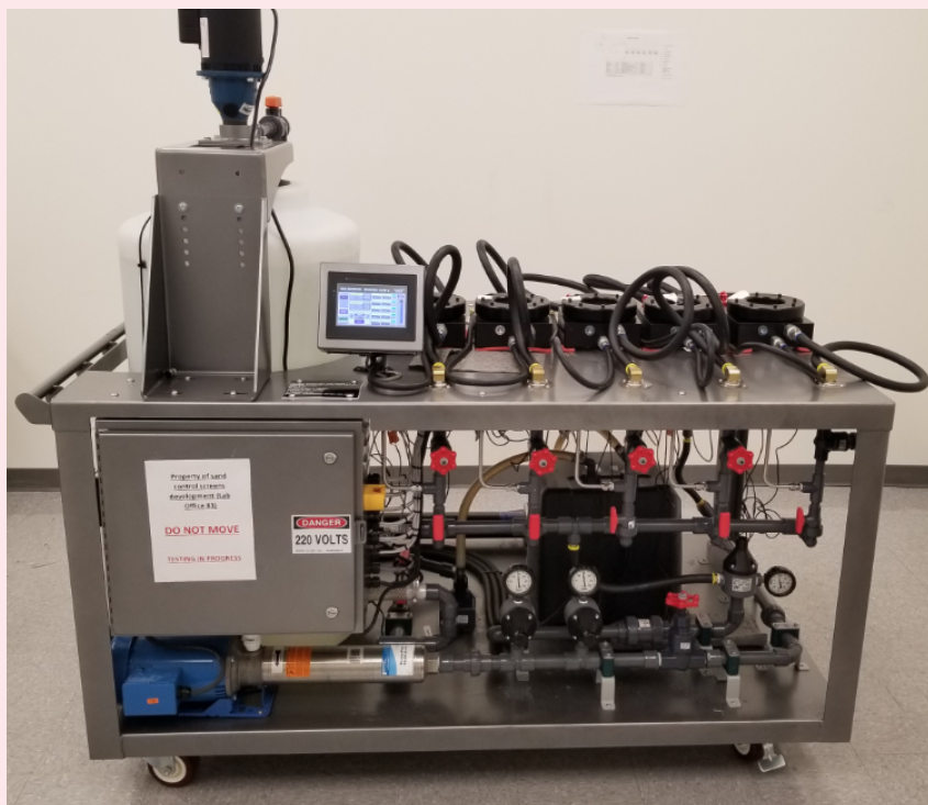
Fig. 12 The additional custom flow loop created for the bearing test flow loop.
