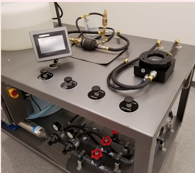
Fig. 11 A custom flow loop was created to perform both system testing and fluid selector testing.
