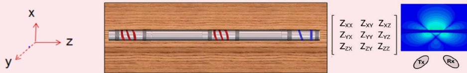
Fig. 4 The ultra-deep resistivity design and measurement components.
