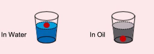
Fig. 3 A float shown in a container of water on the left, and a container of oil on the right; Earth's gravity of 1 g is felt by the float.
