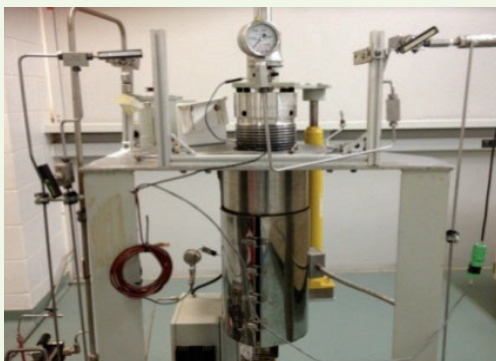
Fig. 6 The high-pressure, high temperature autoclave system used for thermochemical pulse testing.
