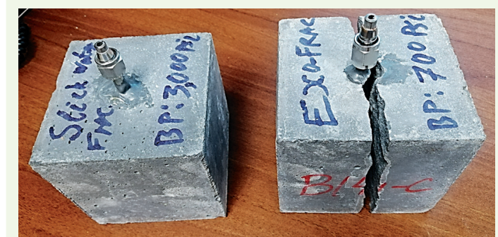
Fig. 16 The impact of thermochemical pulse fracturing on breakdown pressure compared to slick water.
