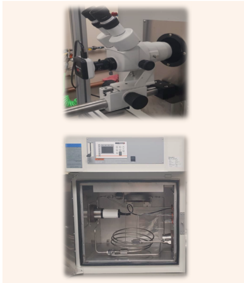
Fig. 2 The class oven includes a flow loop, Coriolis flow meter, view cell, and light bulb assembly.
