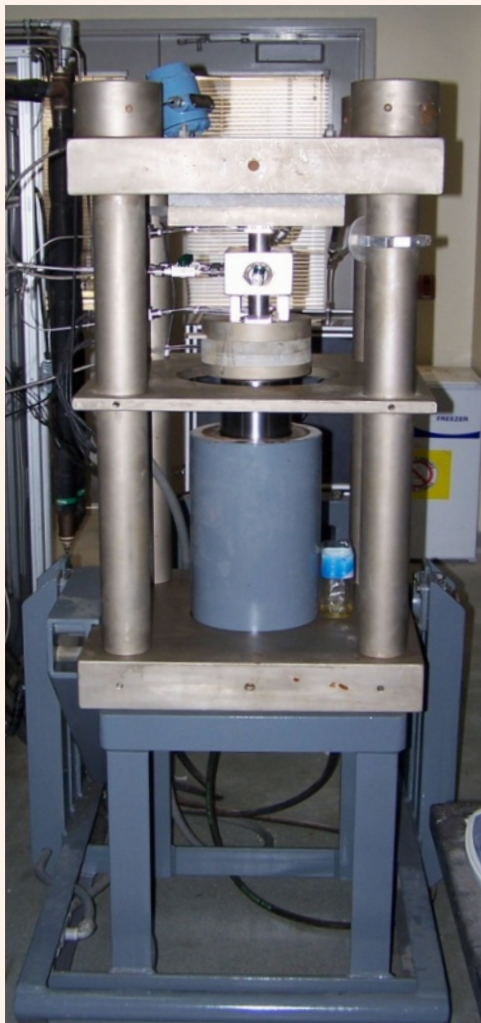
Fig. 4 The used autoclave system, rated up to 20,000 psi and 500 °C.
