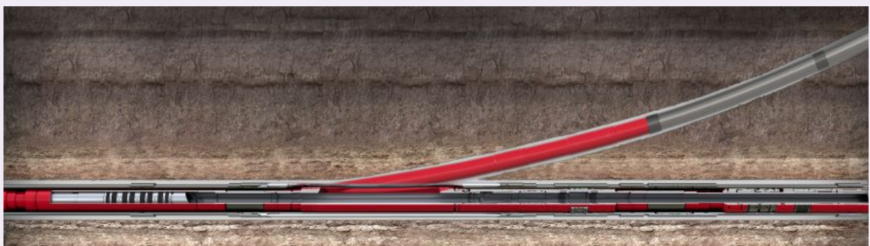
Fig. 17 A pressure isolation sleeve outside the window.
