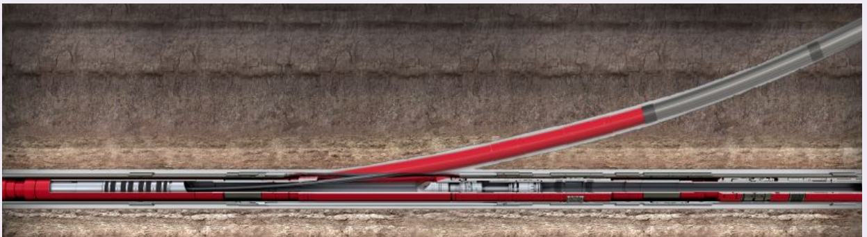
Fig. 20 The wellbore treatment BHA was run inside the lateral.
