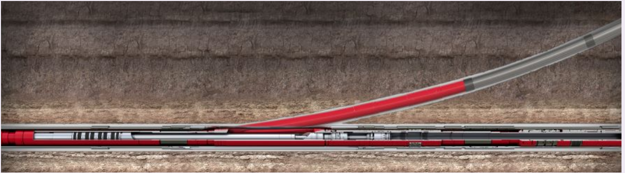
Fig. 18 A TEW run on a slick line and installed in the window.
