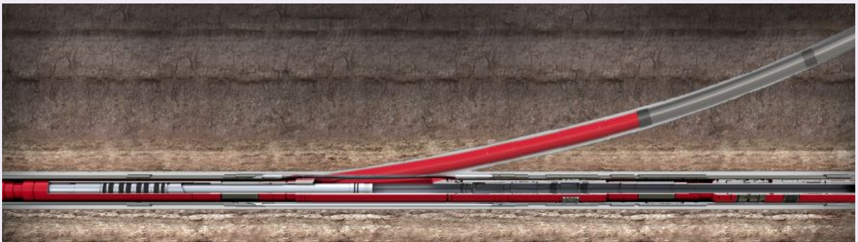
Fig. 16 A pressure isolation sleeve retrieved by a slick line.
