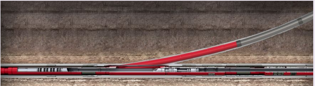
Fig. 19 A TEW installed inside the reentry window.
