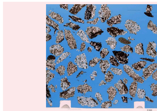
Fig. 7 An example of a thin section HRI of the synthetic cutting sample.
