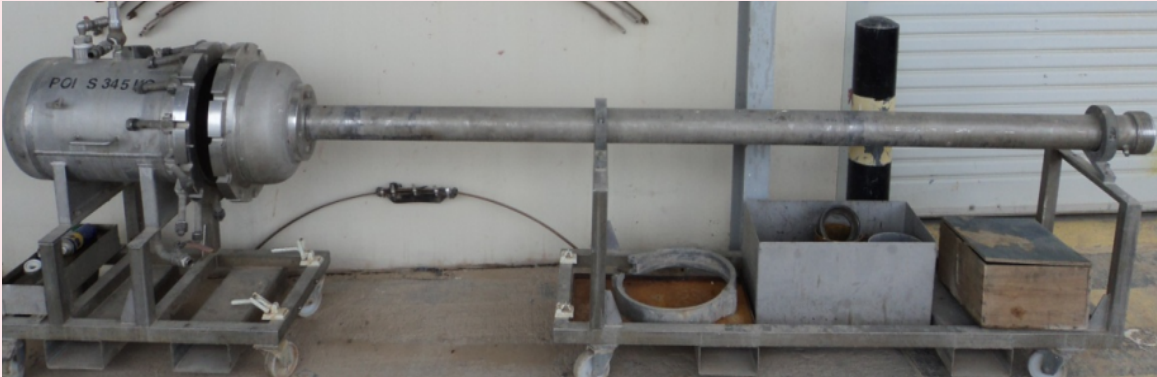
Fig. 3 An image of a tank setup that is used in the controlled testing of the ultrasonic sensor against a casing sample to measure the acoustic impedance.
