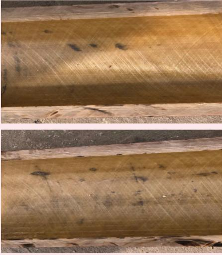
**Fig. 8** The high side of a fiberglass pipe after multifinger caliper logging passes.
