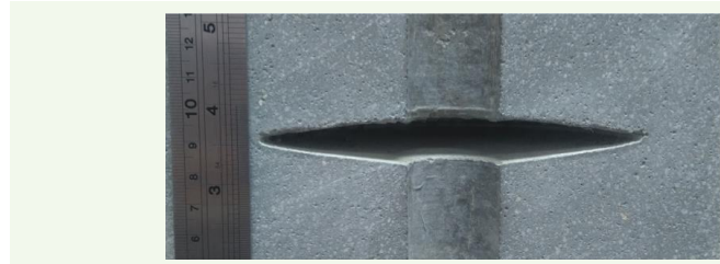
Fig. 9 The dissected section of the trial cement grout block showing the cast borehole and V-shaped circular notch. The borehole and notch are free of wax with only a few visible traces left, which are negligible for experimentation.
