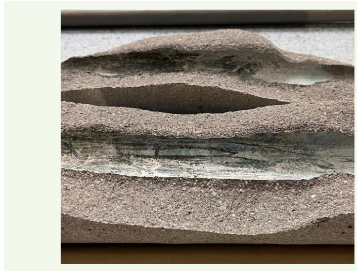
Fig. 12 A closeup photo of the 4" central core extracted from the AUN-002 block (baseline open hole). The core came apart along the longitudinal fracture.
