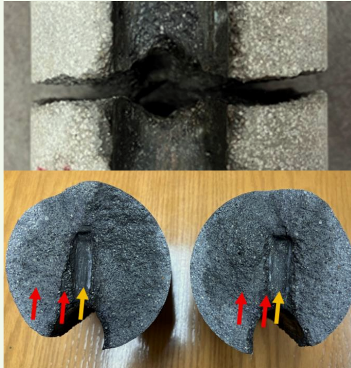
Fig. 13 A closeup photo of the 4" central core extracted from the AUN-004 block (1-hole). The core fell apart along the transverse fracture initiated at the perforation hole.
