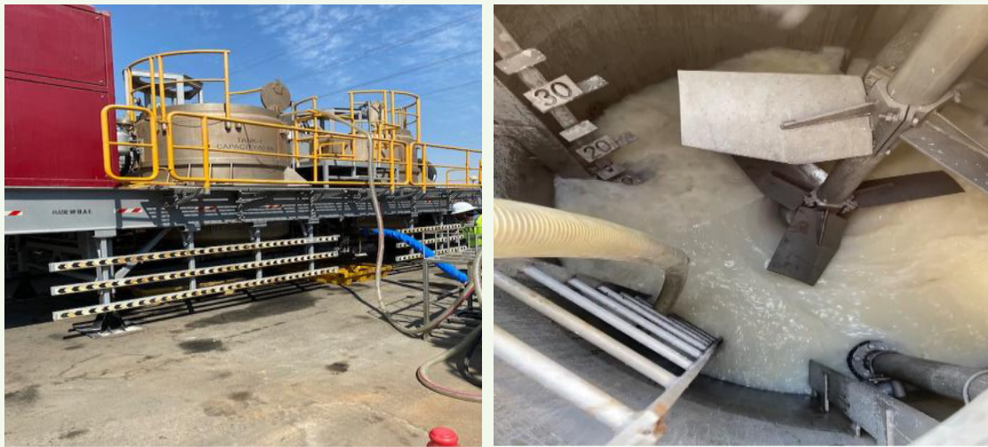
Fig. 7 The actual batch mixer for oil field applications.
