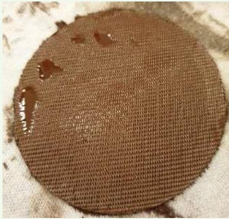
Fig. 13 The 250 \mu screen after the PST.
