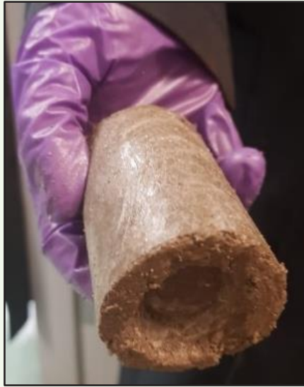
Fig. 1 The epoxy resin-based geopolymer of formulation 3 with a strength of 2,340 psi.
