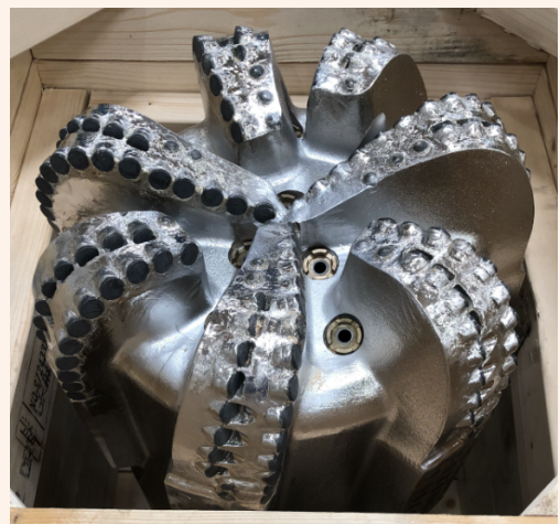
Fig. 7 The metallic anti-balling coating applied on the blades of the drill shoe, behind the cutters 6 .
