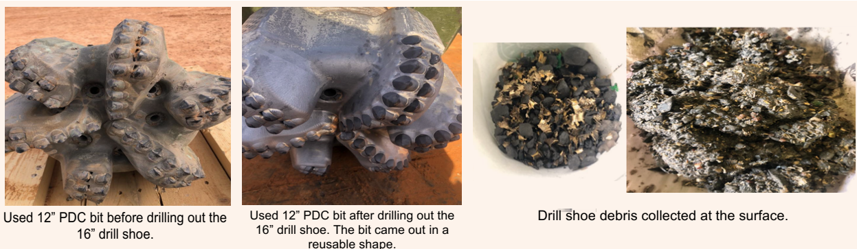
Fig. 16 A comparison between the used 12" conventional bit condition before and after drilling out the 16" cemented in place drill shoe. Also, a picture of the actual debris of the drill shoe collected on the surface.
