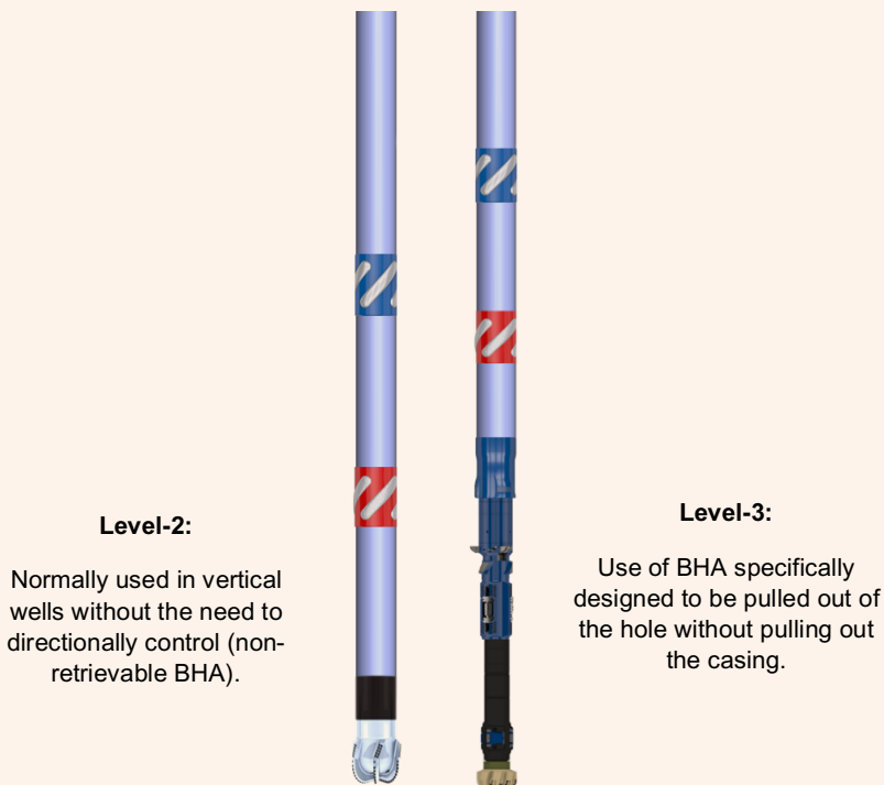
Fig. 3 The commonly used CwD systems. Level-2 was selected for the two wells to drill and case off the trouble zones through sidetracked wellbores 3 .
