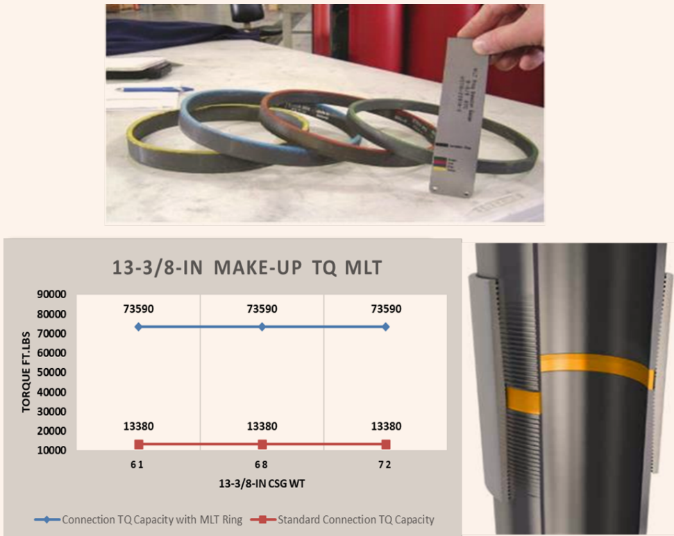
Fig. 8 The different lengths of the multi-torque rings with different color codes, allowing for the small differences in the casing joint's connection lengths. The chart shows the capability to increase the makeup torque strength of the API casing connections.
