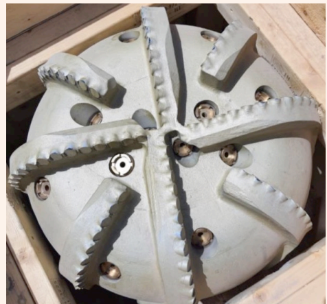
Fig. 19 The used 22" 8-blade bit with 16-mm cutter length with no backup raw drill shoe.
