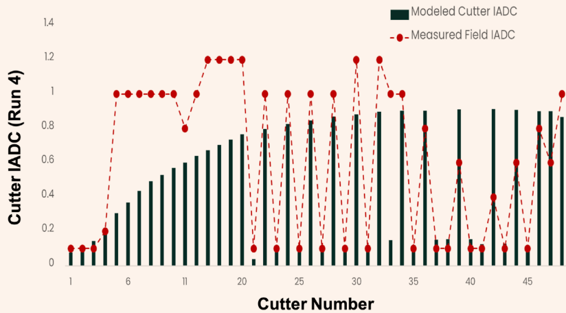
Fig. 5 The detailed model: predicted wear distribution vs. wear distribution on test run 4.
