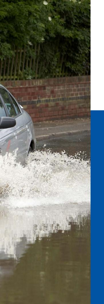
Another hazard is getting stuck while attempting to drive through water. The air intake on most vehicles is low and at the front of the vehicle, and if water enters here the vehicle could stall and may not start again. This could leave you in the dangerous situation of needing to abandon your vehicle and walk in the water.
